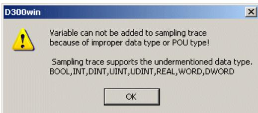
Note 2: Though there is no limit on the number of registered variables, the number of variables that are actually sampled is limit to 10 for one resource. When more than 10 variables are registered, select maximum 10 target variables of sampling, using the following procedure:
