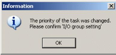
← The confirmation dialog box as shown at left is displayed whenever a task is added or inserted. When a task is added, be sure to confirm or set I/O group in the system definition.
