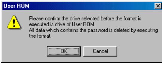
Note) User ROM formatted by WindowsXp/Vista cannot be used with SPH300 CPU version V58 or before. In this case, format using Windows2000.
