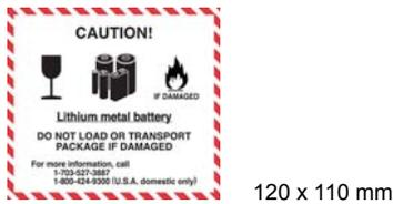
Figure 7.4-4 Label to be Attached to Outer Wrapping
