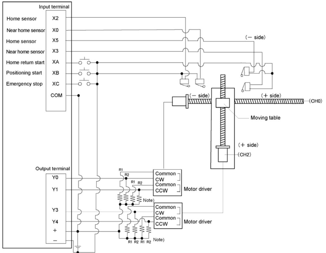
Note) If the input of the stepping motor is 5V photocoupler type, connect a resistor of  $2k\Omega$  (1/2 W) to R1, and connect a resistor of  $2k\Omega$  (1/2 W) –  $470\Omega$  (2 W) to R2.
