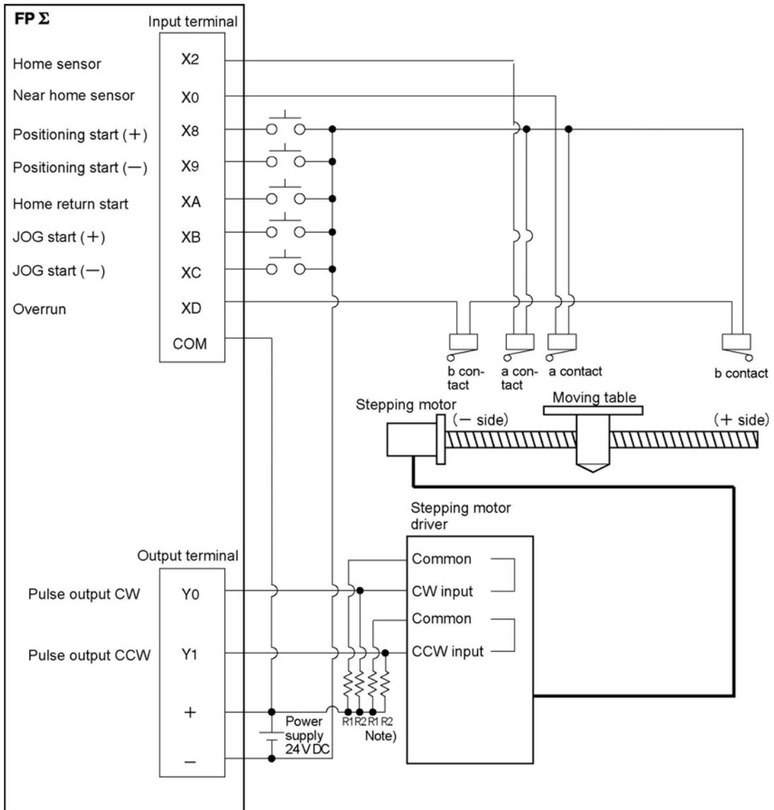
Note) When the stepping motor input is a 5 V optical coupler type, connect a resistor of 2 k $\Omega$  (1/2 W) to R1, and connect a resistor of 2 k $\Omega$  (1/2 W) – 470  $\Omega$  (2 W) to R2.
