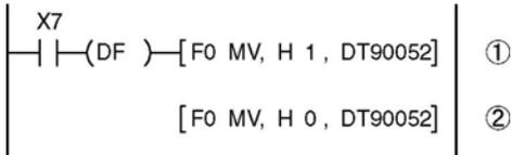
In the above program, the reset is performed in step (1) and 0 is entered just after that in step (2). The count is now ready for operation. If it is only reset, counting will not be performed.
