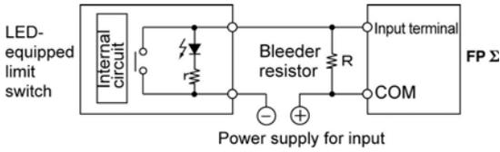
If the input of PLC does not turn off because of the leakage current from the LED-equipped limit switch, the use of a bleeder resistor is recommended, as shown below.
