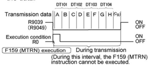
3. When all of the specified quantity of data has been transmitted, the S value is cleared to 0 and the “transmission done” flag R9039/R9049 turns on.
