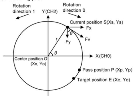
Let CH0 be the X-axis, and CH2 be the Y-axis.
