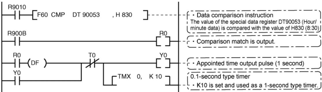
The hour data is stored in the upper 8 bits of DT90053 and the minute data in the lower 8 bits, in the BCD format. This hour and minute data is compared with the appointed time (BCD), and the R900B (=flag) special internal relay is used to detect whether or not it matches the appointed time.
