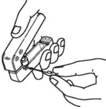
(2) Insert the wire without removing its insulation until it stops, and lightly grip the tool.
