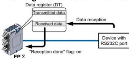
Data input from the COM port is stored in the receive buffer specified by the system register, and the "reception done" flag goes on. If the "reception done" flag is off, data can be received at any time.
