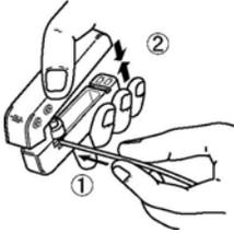
(3) After press-fitting the wire, insert it into the housing.
