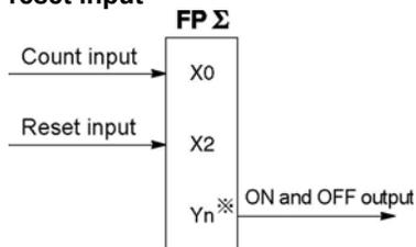
\* The output turned on and off when the target value is reached can be specified from Y0 to Y7 as desired.
