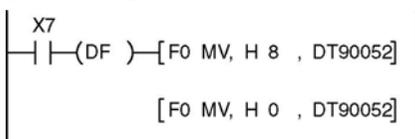
The output counting value of the elapsed value area may be different from the input counting value of the motor side if the forced stop is executed by these programs.
