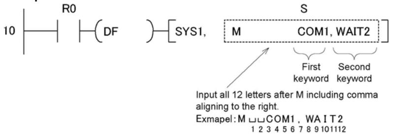
When R0 turns on, the response of COM1 port (RS485 port) delays for two scans. If the scan time is 500μs, it delays for 1 ms.
