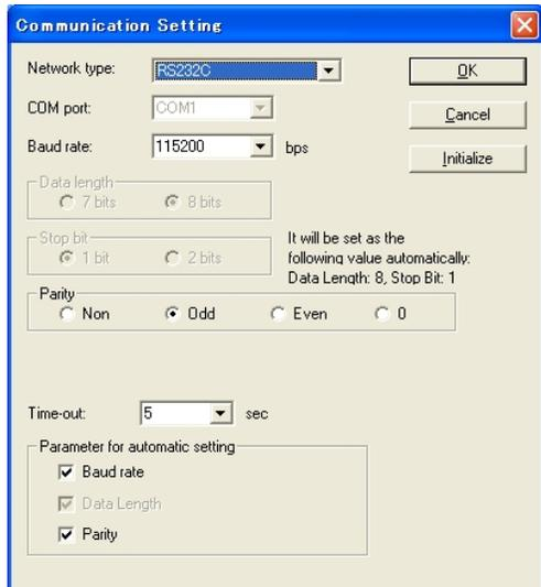
Select "Transfer" from "File" in the menu bar. The "transfer data" screen will open. Select "Condition" to open "Communication Setting" screen. Change the value for "Timeout". Click "OK" button to complete the change of setting.
