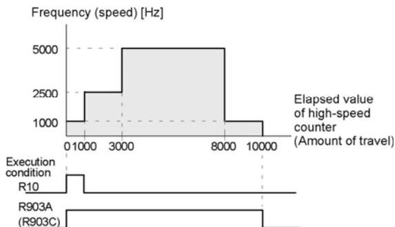
Note) When the execution condition R10 of the F174 (SP0H) instruction goes on, the high-speed counter control flag R903A (R903C) goes on. When the elapsed value reaches 10000 and pulse output stops, R903A (R903C) goes off.
