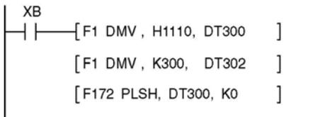
While XB is in the on state, a pulse of 300 Hz is output from Y0.
