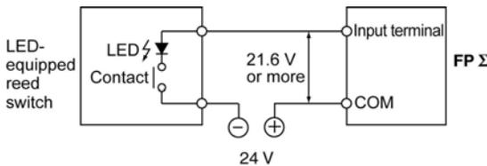
When an LED is connected in series to an input contact such as LED-equipped reed switch, make sure that the on voltage applied to the PLC input terminal is greater than 21.6V DC. In particular, take care when connecting a number of switches in series.
