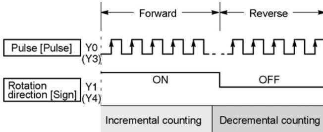
Control is carried out using one pulse output to specify the speed and another to specify the direction of rotation with on/off signals. In this mode, forward rotation is carried out when the rotation direction signals is ON.
