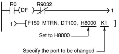
The RS232C port selection flag in R9032 or R9042 turns on when general-purpose serial communication mode is selected.
