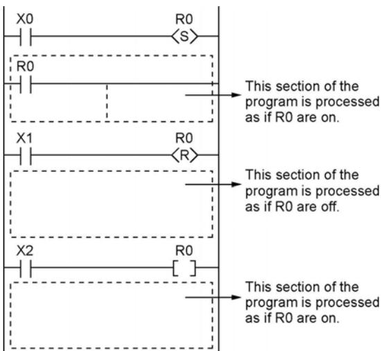
**The output is determined by the final operation results**
