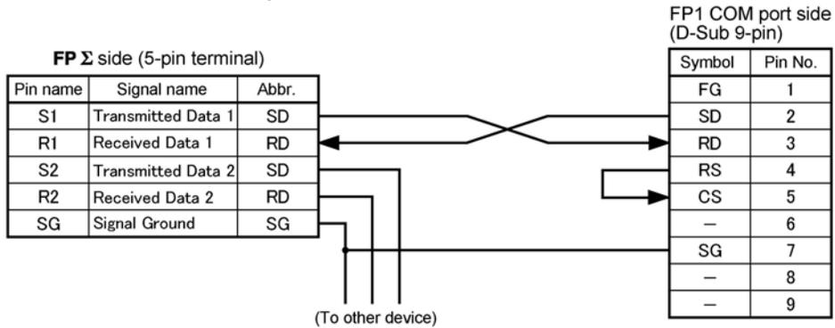
**<Using AFG806, 1-channel RS485 type and 1-channel RS232C type in combination>**
