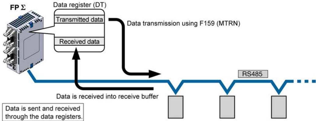
When data has been sent from FPΣ via the RS485 communication of AFPG806, start sending data to FPΣ side after the time mentioned below passed at the receiver.
