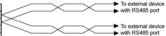
In case of using the AFPG806, connect two cables each to the (+) terminal and (-) terminal. Use the wires of the same cross-sectional area which should be 0.5 to 0.75 mm<sup>2</sup>.
