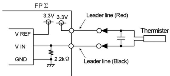
Non-isolated between the FPΣ thermister input unit and the power supply connector (24V).
