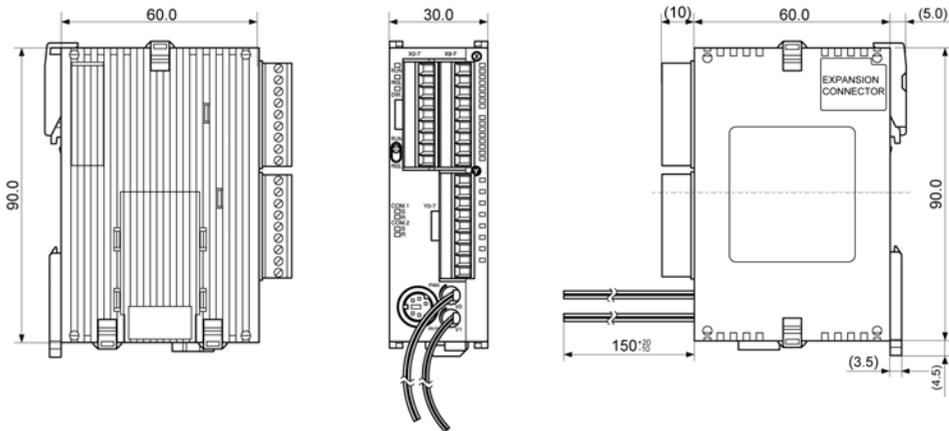
\* The dimension with the communication cassette mounted is the same as the transistor output type.
