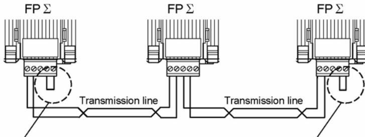
The final unit (terminal station) should be shorted between the transmission line (-) and the E terminal.
