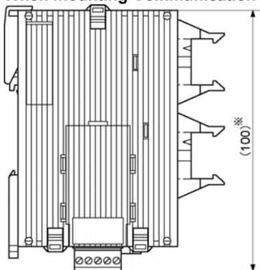
\* The dimension with the communication cassette mounted is 105mm.
