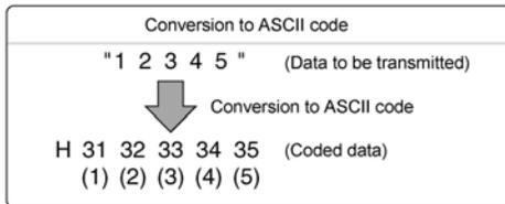
2. If DT100 is being used as the send buffer, data will be stored in sequential order in the data registers starting from the next register (DT101), in two-byte units consisting of the upper and the lower byte.
