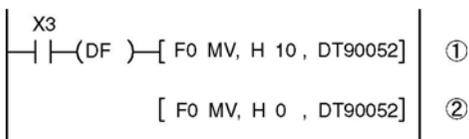
In these programs, the near home input is enabled in step (1) and 0 is entered just after that in step (2) to perform the preset operations.
