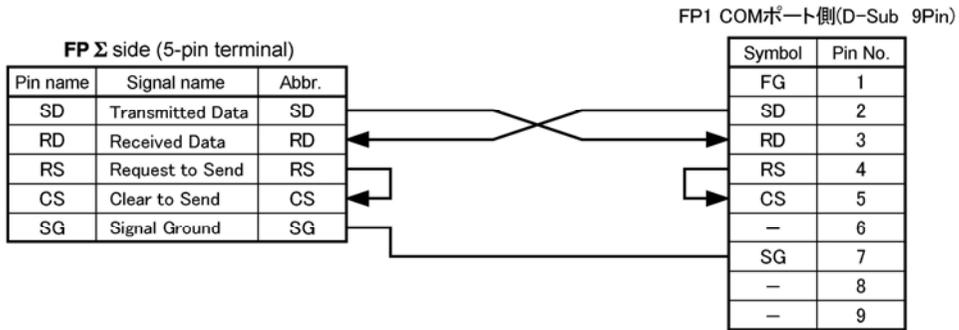
**<Using AFPG802, 2-channel RS232C type communication cassette>**
