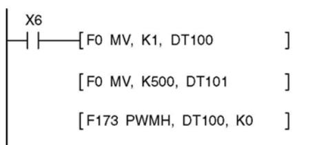
While X6 is in the on state, a pulse with a period of 502.5 ms and duty ratio of 50% is output from Y0 of specified channel "CH2".
