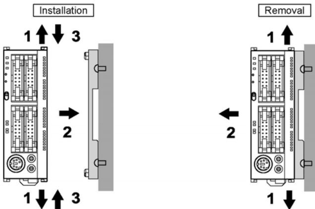
An unit with an attached flat type mounting plate can also be installed sideways on a DIN rail.
