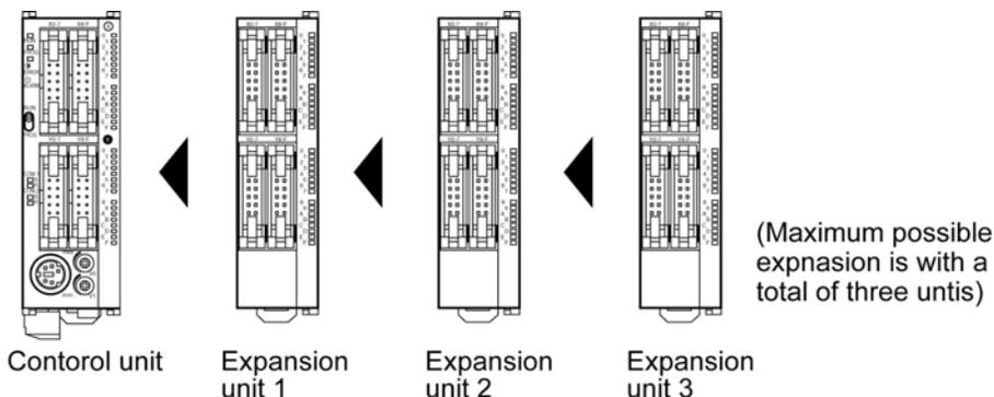
Up to three expansion units can be added on the right of the FPΣ, these expansion units being either expansion units or intelligent units from the earlier FP0 series, or a combination of the two. A combination of relay output types and transistor output types is also possible.
