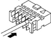
(4) When all wires has been inserted, fit the semi-cover into place.
