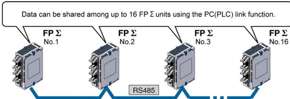
**PC(PLC) link function (up to 16 units) or 1:N communication (up to 99 units) with RS232C devices**
