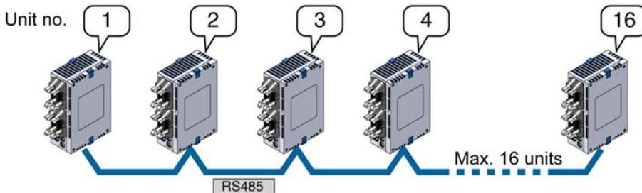
Unit numbers are the numbers to identify the different PLCs on the same network. The same number must not be used for more than one PLC on the same network.
