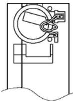
Note) When replacing the battery, turn off the power after supplying the power more than 1 min., and then fit the new battery within 2 min of removing the old one.
