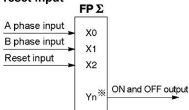
\* The output turned on and off when the target value is reached can be specified from Y0 to Y7 as desired.
