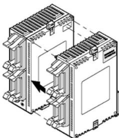
**(4) Press down the expansion hooks raised in step 2 to secure the unit.**
