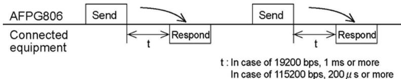
**Following adjustments are required depending on the types of connected equipment.**
