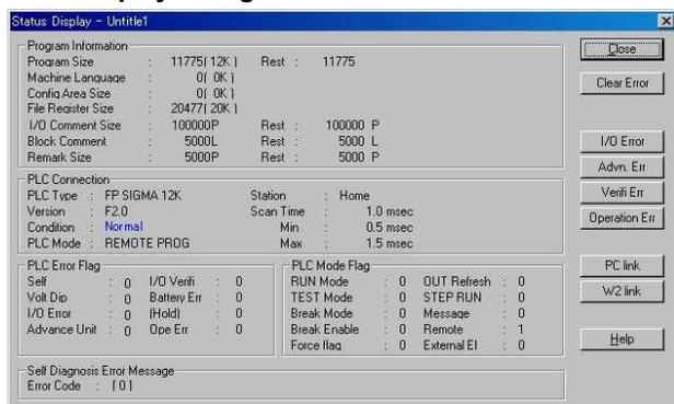
If the error is an operation error, the error address can be confirmed in this dialog box.
