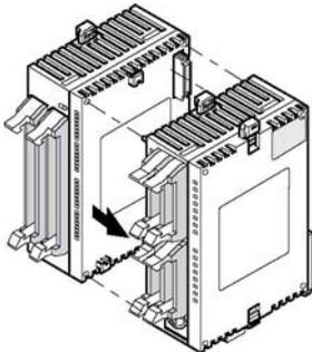
**(4) Press down the expansion hooks raised in step 2 to secure the unit.**
