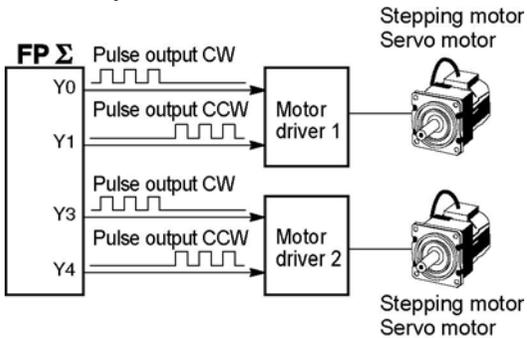
Combined with a commercially available motor driver, the function enables positioning control. With the exclusive instruction, you can perform trapezoidal control, home return, and JOG operation.
