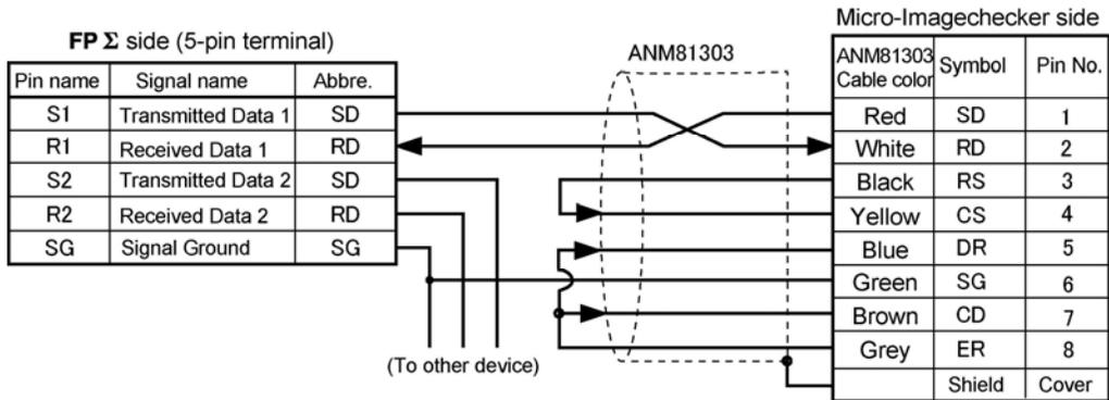
**<Using AFPG806, 1-channel RS485 type and 1-channel RS232C type in combination>**
