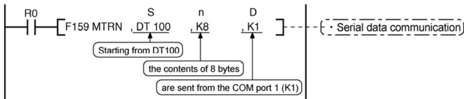
**Devices that can be specified for S:** Only data registers (DT) can be specified as the send buffer.
